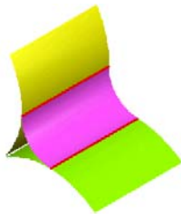
Extract Curves from the Fillet Surface Edges Using Extract Curve Tool
